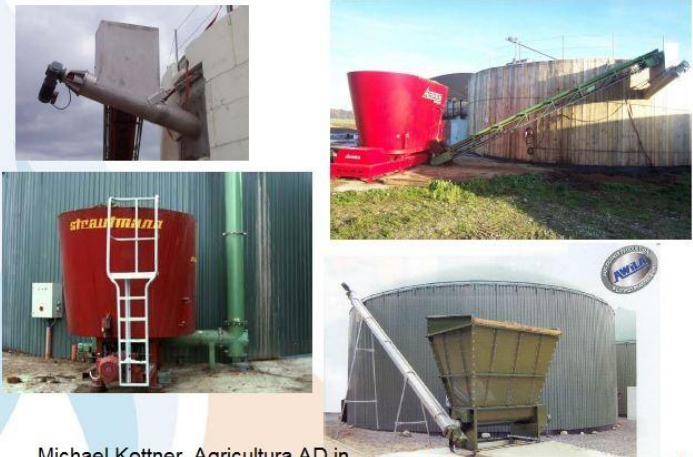
Direct feeding of solid biomass
