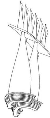
Figure 3. Fork-shaped blade of two-tier stage.
