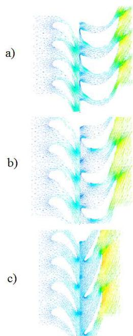
Figure 5. Velocity fields in lower tier of two-tier stage.
