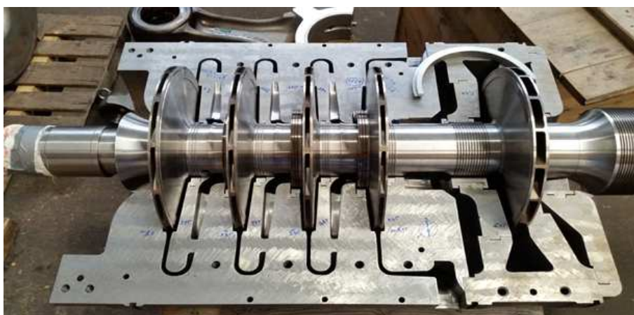
Figure 4: HP section of the modernized machine.
