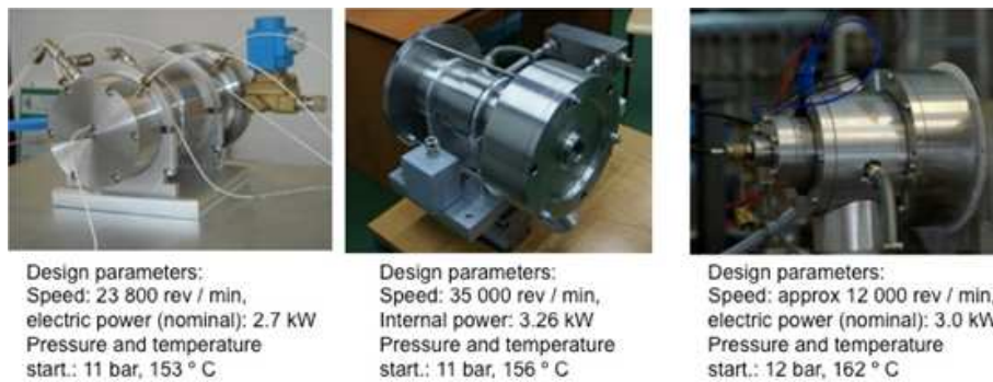
Figure 4: Domestic Micro-CHP ORC Unit. Microturbines: developed target versions. Elaborated in TU Łódź and TU Gdańsk in cooperation with IMP PAN. Two pictures on the left: radial and supersonic microturbine; picture on the right: axial microturbine.
