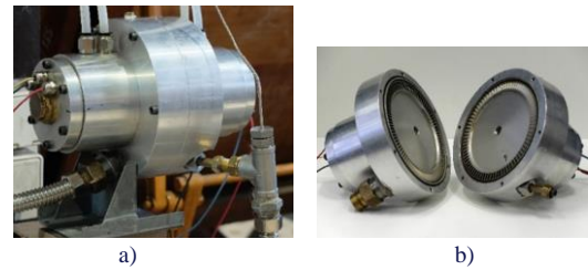
Fig. 5. View of a steam microturbine with two generators (a) and both counter-rotating rotors in separate housings (b).
