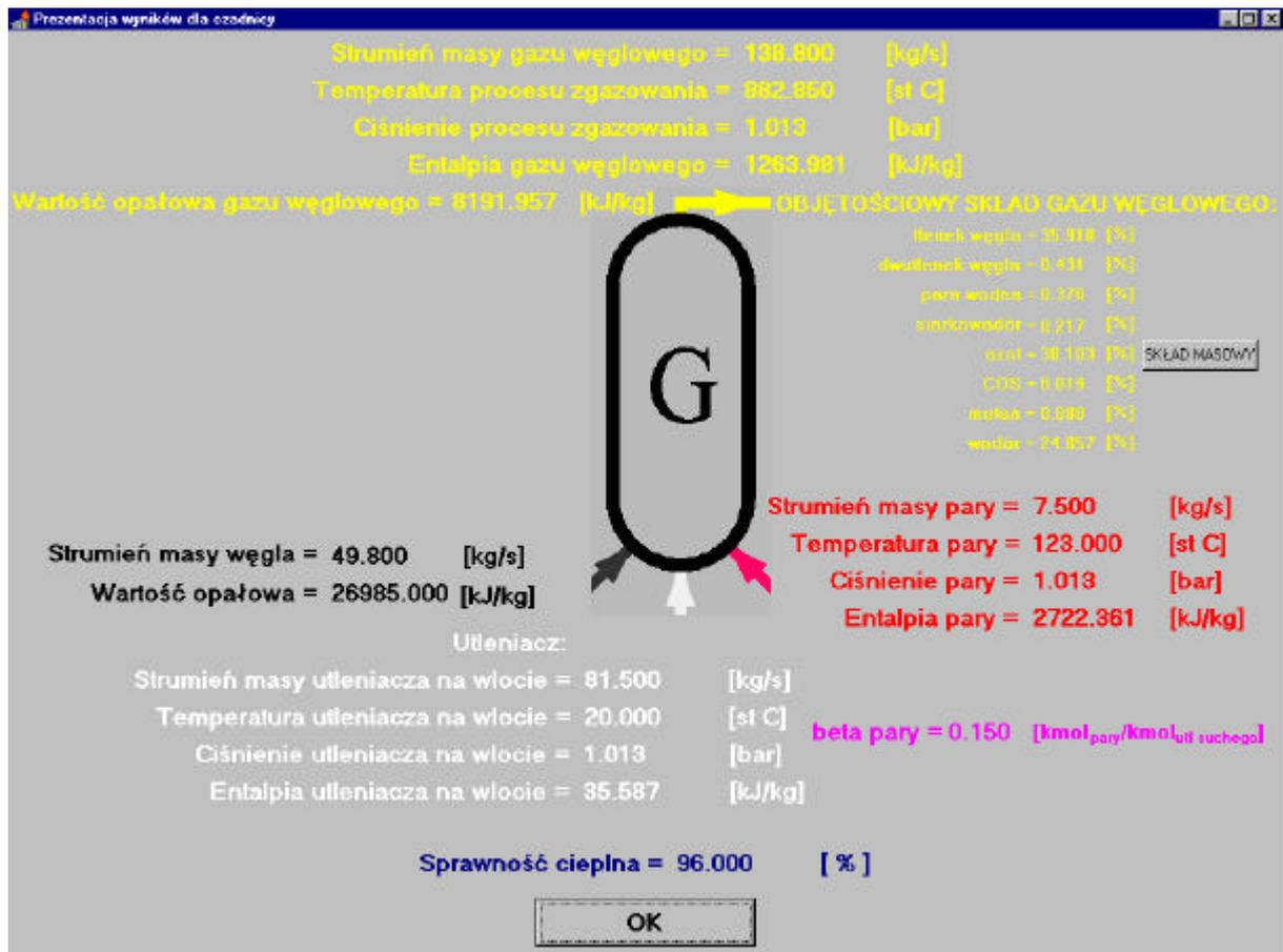
FIGURE 3. Typical results presentation in the COM-GAS code [19].
