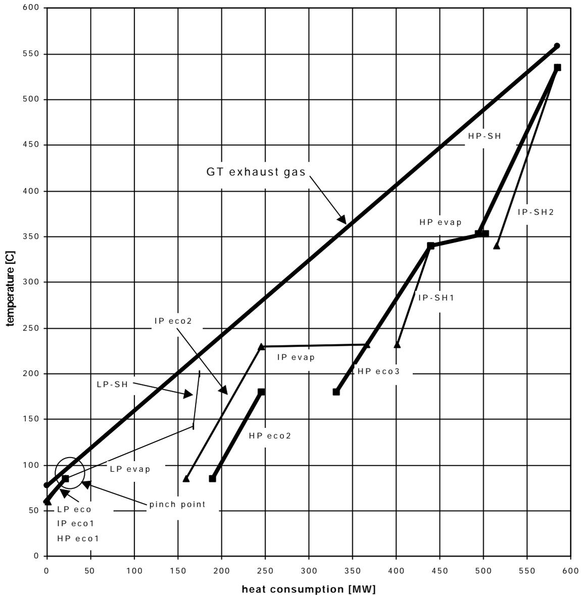
FIGURE 4. Heat consumption versus temperature diagram for the HRSG
