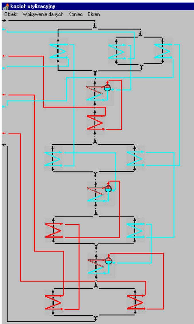
Figure 2. Scheme of a triple-pressure HRSG
