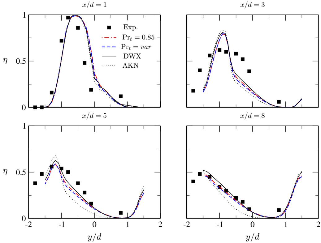
Figure 4. Cooling effectiveness for velocity ratio  $VR = 0.5$
