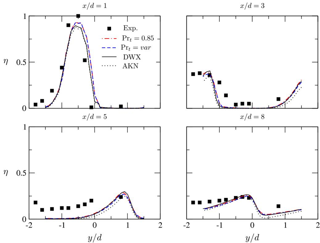
Figure 6. Cooling effectiveness for velocity ratio  $VR = 1.5$
