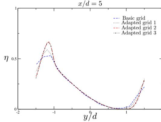
Figure 3. Cooling effectiveness  $\eta$  at the cross-section  $x/d = 5$  after subsequent grid adaption
