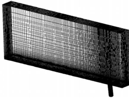
Figure 2. Computational grid for flat plate cooling
