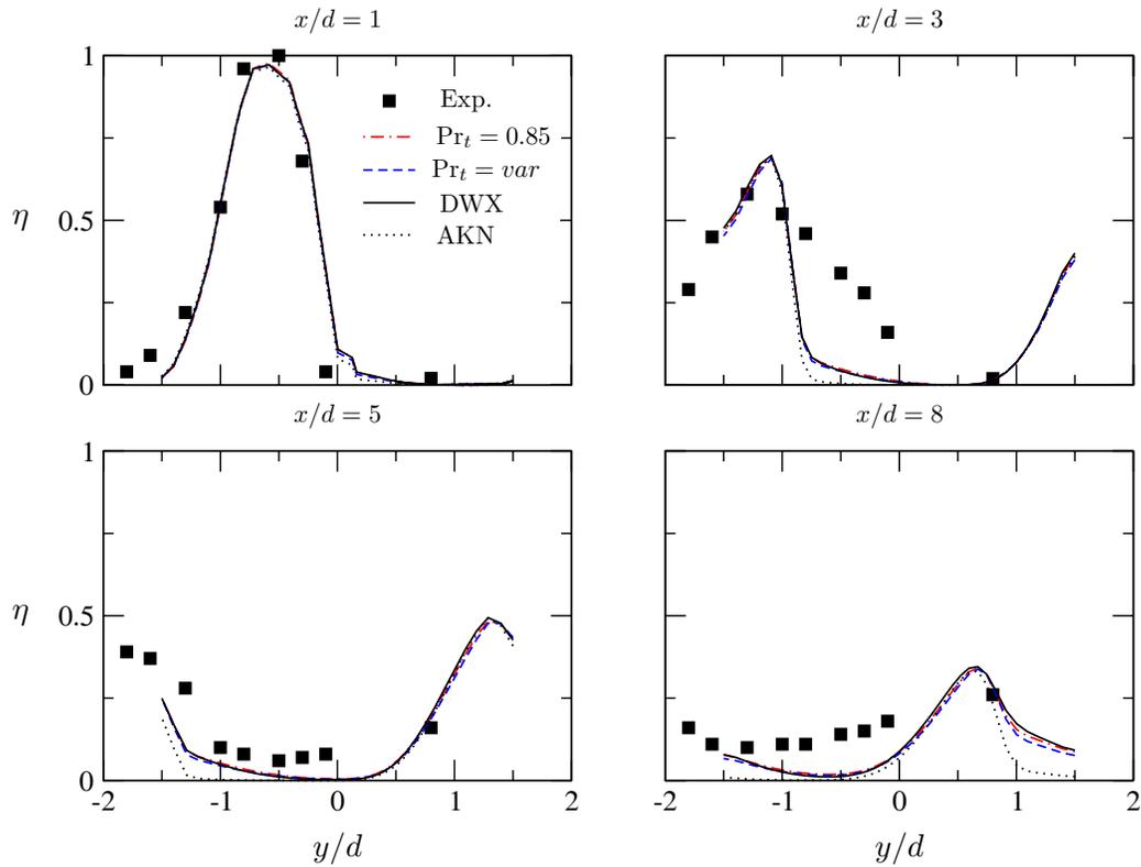
Figure 5. Cooling effectiveness for velocity ratio  $VR = 1.0$
