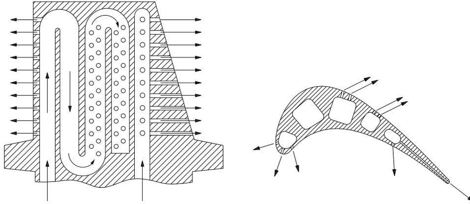
Figure 1. Internal and external cooling systems [2]
