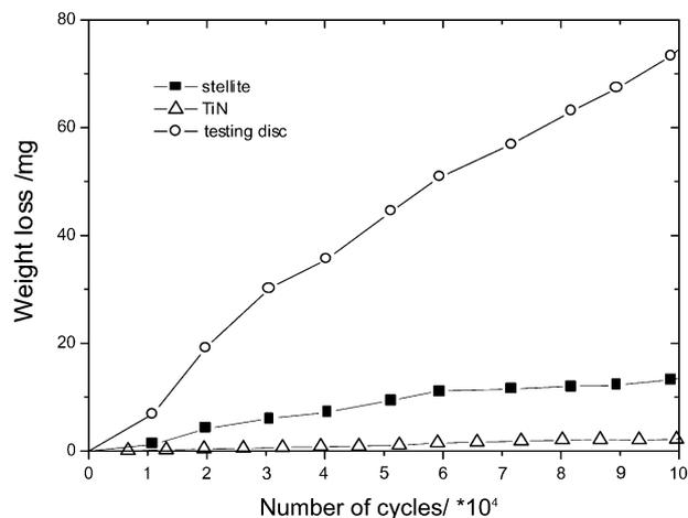
Fig. 5. The wear resistance as a dependence of the weight loss due to friction on the test duration; experimental data refer to the stellite (squares), and to the testing disc (circles); the data of TiN (triangles), are given for reference only.
