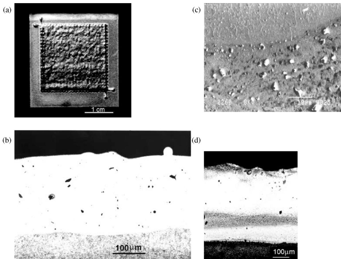
Fig. 2. (a–d) Photographs of the sample structure: a general view of the stellite coating of dimensions  $20 \times 20 \times 0.7 \text{ mm}^3$  (a); cross-section of a single-layer coating (b); SEM micrograph of the dendritic structure of the stellite (upper zone) and the structure of the substrate; the interface and also white precipitates are clearly observed (c); and a cross-section of a stellite clad, total height of two layers = 0.7 mm, magnification (d).
