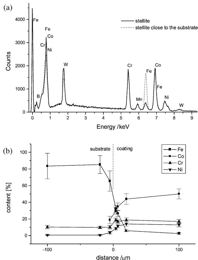
Fig. 3. (a,b) Semi-quantitative EDS data on the dominant chemical components of the bulk stellite—full line, and of its region close to the base material—dashed line (a); dependence of the relative content (%wt.) of constituents Fe, Co, Cr, and Ni on the distance from the substrate–clad interface (b).
