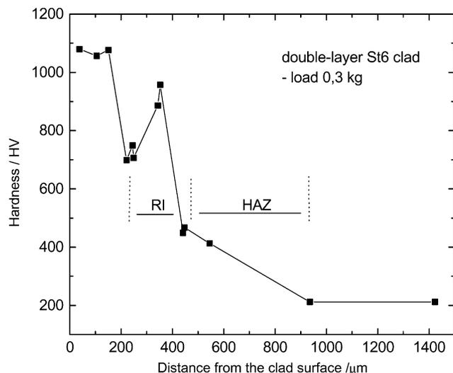
Fig. 4. The dependence of the Vickers microhardness on the distance from the top surface of the coating; marked are the remelted interlayer (RI) and heat affected (HAZ) zones, data correspond to the sample shown in Fig. 2d.
