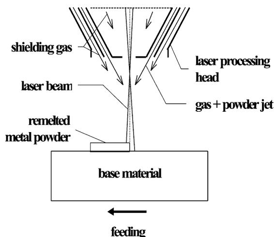
Fig. 1. The axially-symmetric experimental setup applied for the laser cladding of stellite powder.
