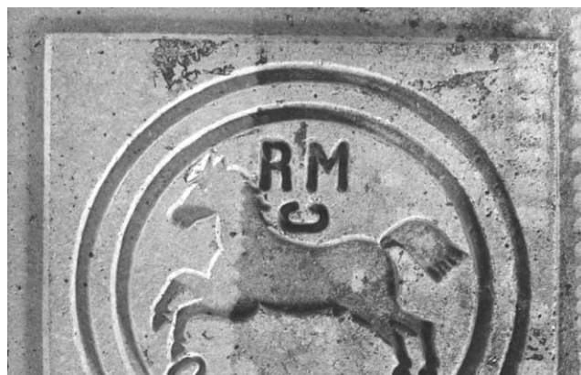
Fig. 1. Surface of the test sample wet cleaned by means of laser ablation: Nd:YAG laser, 1064 nm, 6 ns pulse duration.
