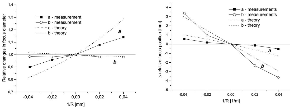
Fig.4 Focus shift and relative changes in the focus size vs radius of curvature of the variable focal length mirror. The measured values are given in relation to the focused beam waist position and its size for the flat mirror; a – the mirror located at the distance of  $0.3\text{m}$  from the laser output window, b - the mirror located at the distance of  $0.2\text{m}$  from the focusing lens and  $4.2\text{m}$  from the laser output
