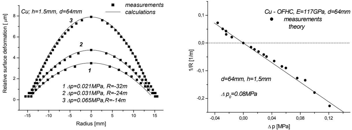
Rys3 2D–contour of the mirror surface resulting from the interferometer measurement (a), the dependence of the curvature radius on the deforming pressure measured in relation to the atmospheric pressure (b)
