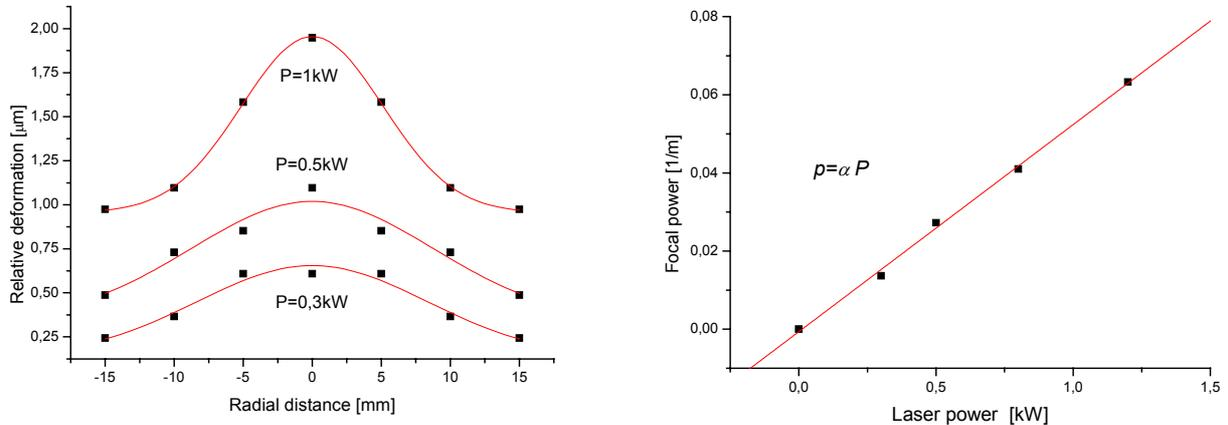
Fig.2 Relative distribution of the deformation of the ZnSe output window as a function of the irradiated power (a), the focal power of thermal lensing in the ZnSe plate as a function of the incident laser power (b)
