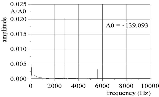
Figure 3a. Amplitude-frequency characteristics for the unsteady modal aerodynamical forces (of the 1<sup>st</sup> mode) up to 10000 Hz
