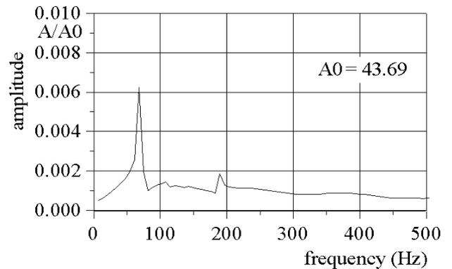
Figure 3d. Amplitude-frequency characteristics for the unsteady modal aerodynamical forces (of the 2<sup>nd</sup> mode) up to 500 Hz
