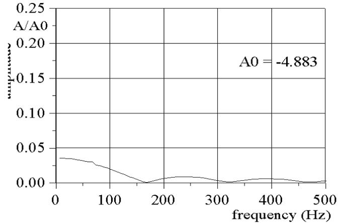
Figure 4b. Amplitude-frequency characteristics for the unsteady modal aerodynamical forces (of the 6<sup>th</sup> mode) up to 500 Hz
