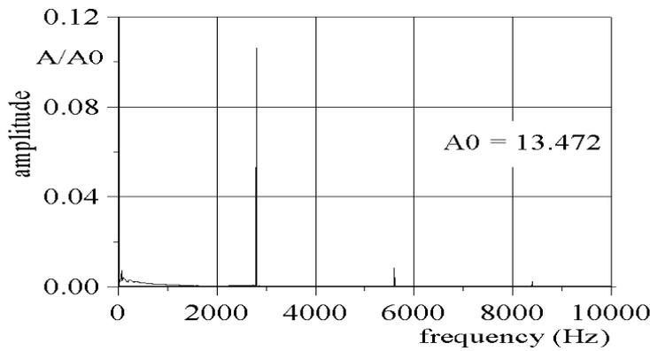
Figure 4e. Amplitude-frequency characteristics for the unsteady modal aerodynamical forces (of the 10<sup>th</sup> mode) up to 10000 Hz
