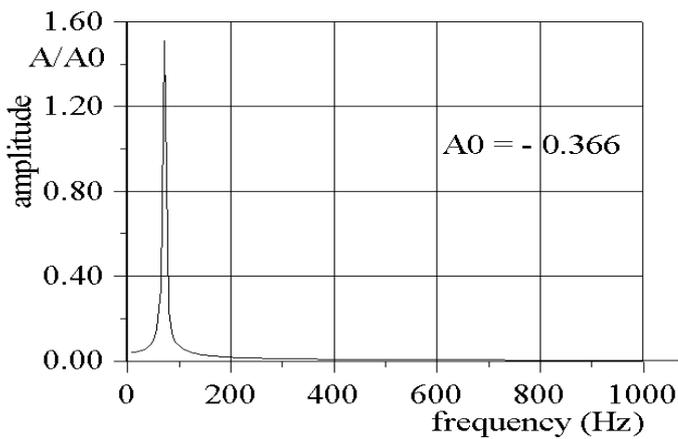
Figure 6a. Amplitude-frequency characteristics for 1<sup>st</sup> blade motion corresponding to 1<sup>st</sup> mode shape
