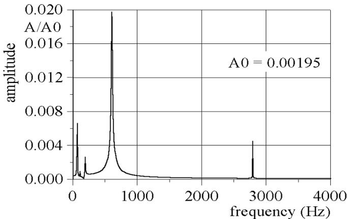
Figure 6f. Amplitude-frequency characteristics for 1<sup>st</sup> blade motion corresponding to the 8<sup>th</sup> mode
