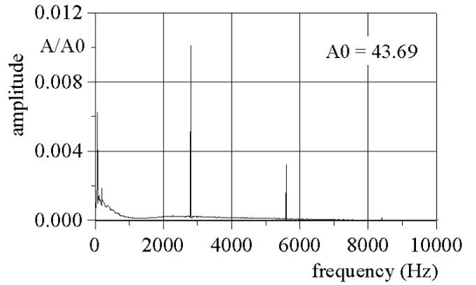
Figure 3c. Amplitude-frequency characteristics for the unsteady modal aerodynamical forces (of the 2<sup>nd</sup> mode) up to 10000 Hz
