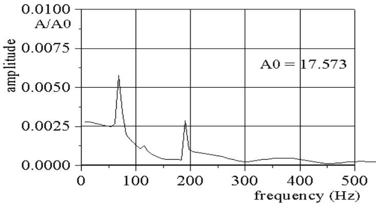
Figure 4d. Amplitude-frequency characteristics for the unsteady modal aerodynamical forces (of the 8<sup>th</sup> mode) up to 500 Hz
