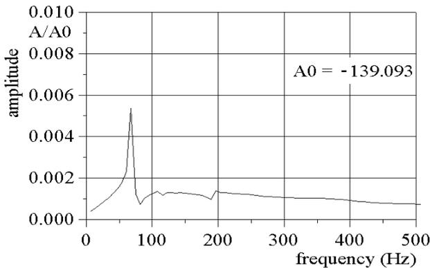
Figure 3b. Amplitude-frequency characteristics for the unsteady modal aerodynamical forces (of the 1<sup>st</sup> mode) for frequency range up to 500 Hz
