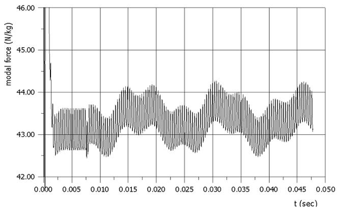
Figure 2c. The unsteady modal forces of 1<sup>st</sup> blade corresponding to 2<sup>nd</sup> mode shape during one rotor rotation
