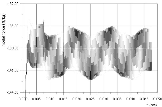
Figure 2b. The unsteady modal force of 5<sup>th</sup> blade corresponding to 1<sup>st</sup> mode shape during one rotor rotation
