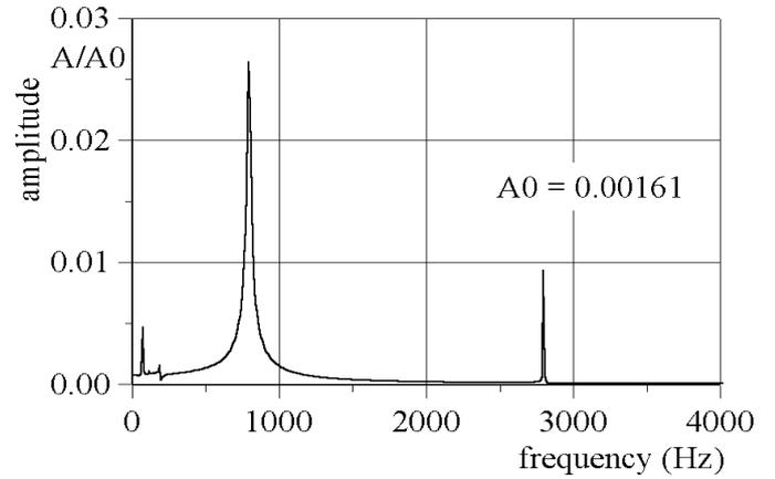
Figure 6g. Amplitude-frequency characteristics for 1<sup>st</sup> blade motion corresponding to 10<sup>th</sup> mode
