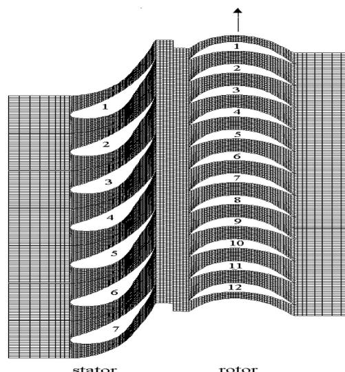
Figure 1a. The tangential section of the turbine stage
