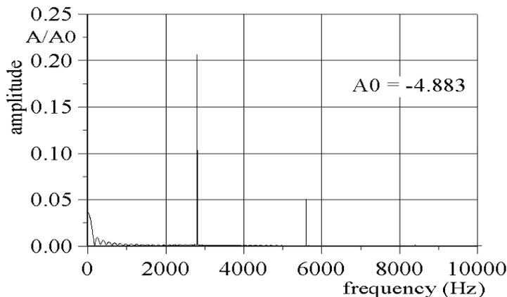
Figure 4a. Amplitude-frequency characteristics for the unsteady modal aerodynamical forces (of the 6<sup>th</sup> mode) up to 10000 Hz
