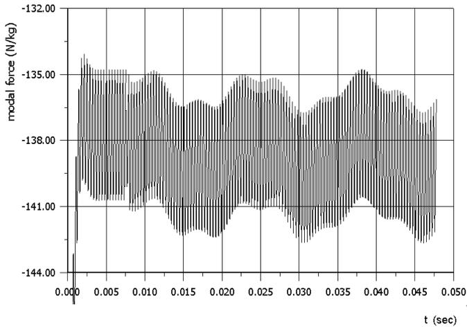
Figure 2a. The unsteady modal forces of the 1<sup>st</sup> blade corresponding to 1<sup>st</sup> mode shape, during one rotor rotation
