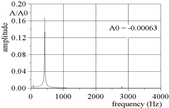
Figure 6e. Amplitude-frequency characteristics for 1<sup>st</sup> blade motion corresponding to 6<sup>th</sup> mode
