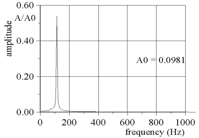
Figure 6b. Amplitude-frequency characteristics for 1<sup>st</sup> blade motion corresponding to the 2<sup>nd</sup> mode
