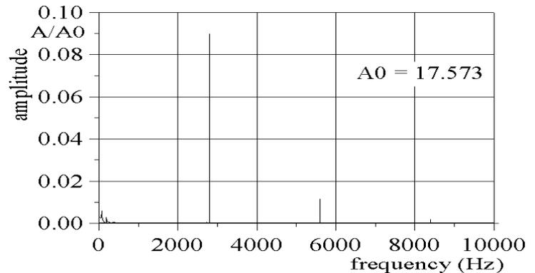
Figure 4c. Amplitude-frequency characteristics for the unsteady modal aerodynamical forces (of the 8<sup>th</sup> mode) up to 10000 Hz
