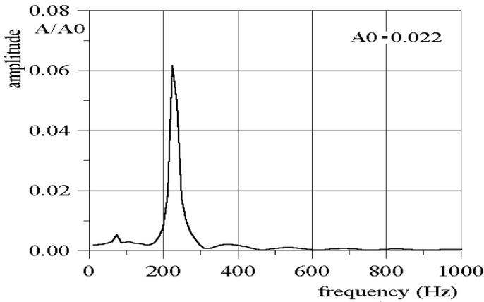
Figure 6d. Amplitude-frequency characteristics for 1<sup>st</sup> blade motion corresponding to the 4<sup>th</sup> mode
