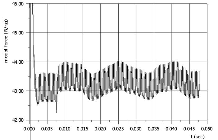
Figure 2d. The unsteady modal forces of 5<sup>th</sup> blade corresponding to 2<sup>nd</sup> mode shape during one rotor rotation
