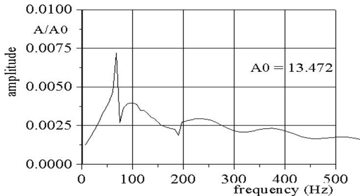
Figure 4f. Amplitude-frequency characteristics for the unsteady modal aerodynamical forces (of the 10<sup>th</sup> mode) up to 500 Hz
