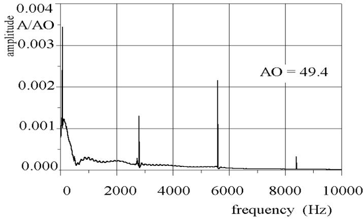
Figure 3g. Amplitude-frequency characteristics for the unsteady modal aerodynamical forces (of the 4<sup>th</sup> mode) for frequency range up to 10000 Hz
