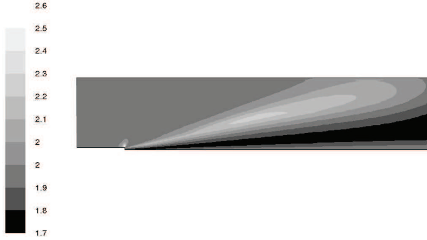
Figure 2. Local changes of C_{\epsilon 2 P o p e} in the axisymmetric coflowed jet.
