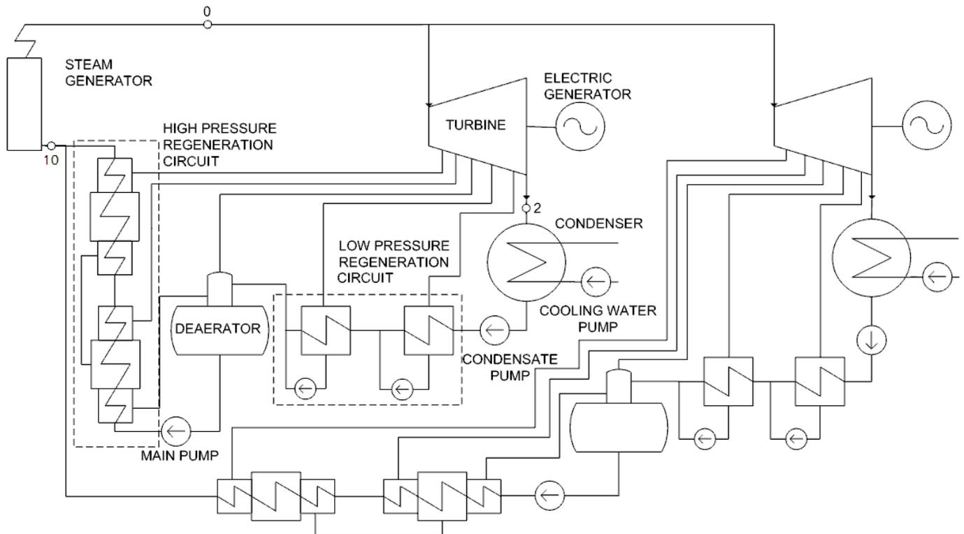
Fig. 1. The twin cycle thermodynamic scheme
