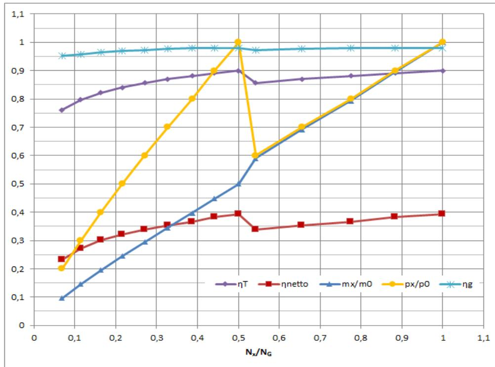
Fig. 4. Characteristic of: electric generators efficiency  $\eta_G$ , electric net efficiency  $\eta_{netto}$ , turbines average mechanical efficiency  $\eta_T$ , and live steam mass flow rate  $m_x/m_0$  as a function load variations  $N_x/N_G$  for cycle with steam reheat.
