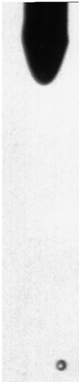
Fig.2. Microdripping mode
