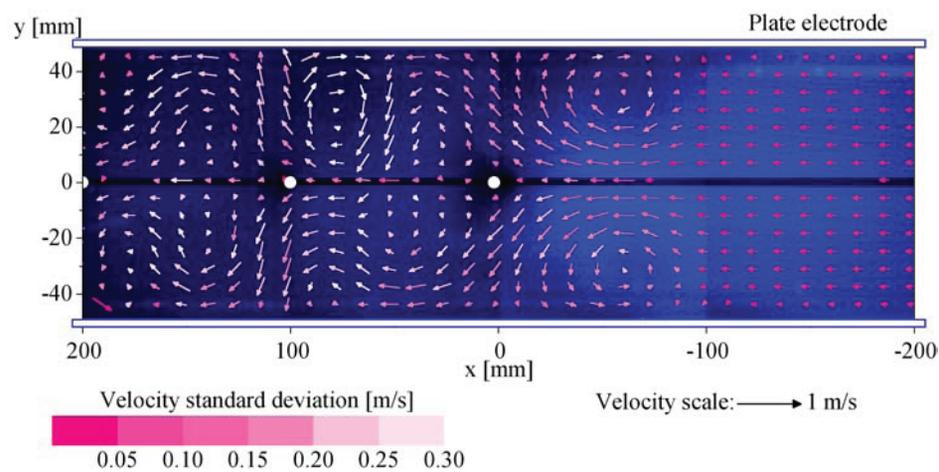
Fig. 5. Flow velocity field in the ESP model at a primary flow velocity of 0.14 m/s. Positive polarity, voltage 24 kV,  $Re = 460$ ,  $N_{EHD} = 28$ . Only the flow patterns around three wire electrodes are shown (on the left side of the third wire electrode, the seed particles vanished due to efficient electrostatic precipitation).
