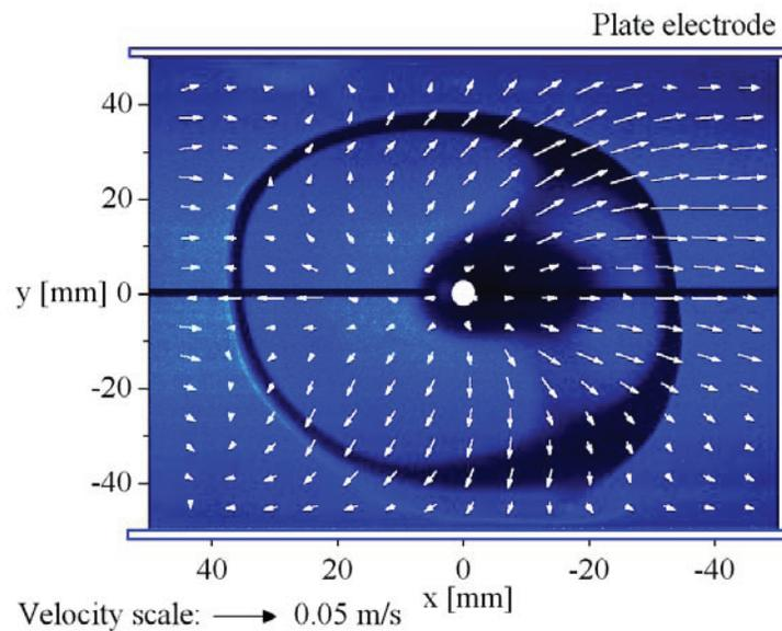
Fig. 3. Image of the seed particle flow pattern and velocity field around the second wire electrode in the ESP model without primary flow at  $t = 1$  s after applying the high voltage. Positive polarity, voltage 17 kV.
