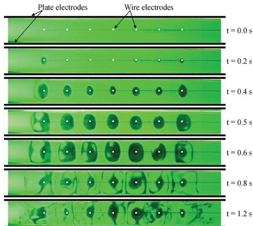
Fig. 2. CuBr laser visualization. Time evolution of the circular structures of the seed particle flow after applying high voltage at  $t = 0$  without primary flow. Positive polarity, voltage 25 kV.
