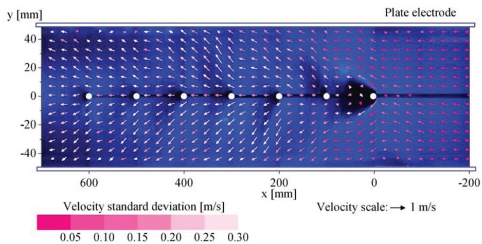
Fig. 6. Flow velocity field in the ESP model at a primary flow velocity of 0.6 m/s. Positive polarity, voltage 24 kV,  $Re = 2000$ ,  $N_{EHD} = 1.7$ .
