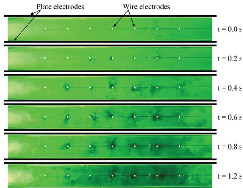
Fig. 4. CuBr laser visualization. Time evolution of the circular patterns of the seed particle flow after applying the high voltage at  $t = 0$  s without primary flow. Negative polarity, voltage 25 kV.
