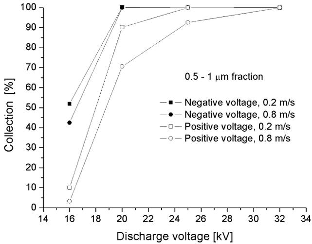
Fig. 1. Percentage of the precipitated submicron particles (0.5–1  $\mu\text{m}$  fraction) as a function of discharge voltage for primary flow velocities of 0.2 and 0.8 m/s. Negative and positive polarity.
