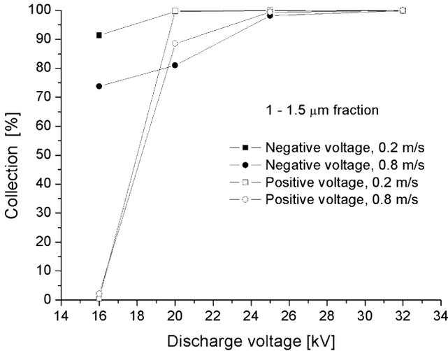
Fig. 2. Percentage of the precipitated 1–1.5  $\mu\text{m}$  particles as a function of discharge voltage for primary flow velocities of 0.2 and 0.8 m/s. Negative and positive polarity.
