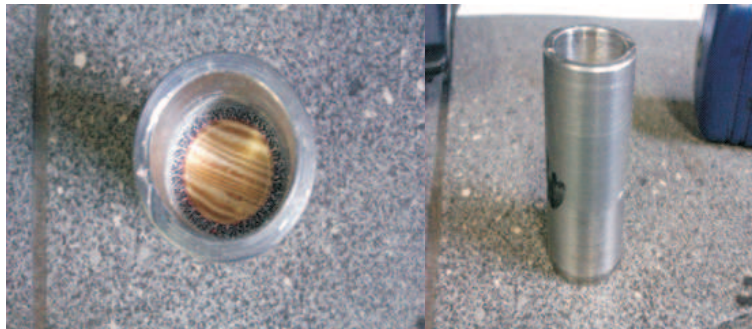
Figure 3: Interchangeable steel sleeve with biomass (pine) samples for permeability measurements.
