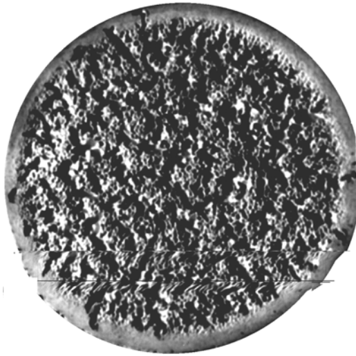
Fig.8 Aluminium specimen after a 120 min test at the vibratory rig of the University of Hiroshima (specimen size: \varnothing 16 mm).
