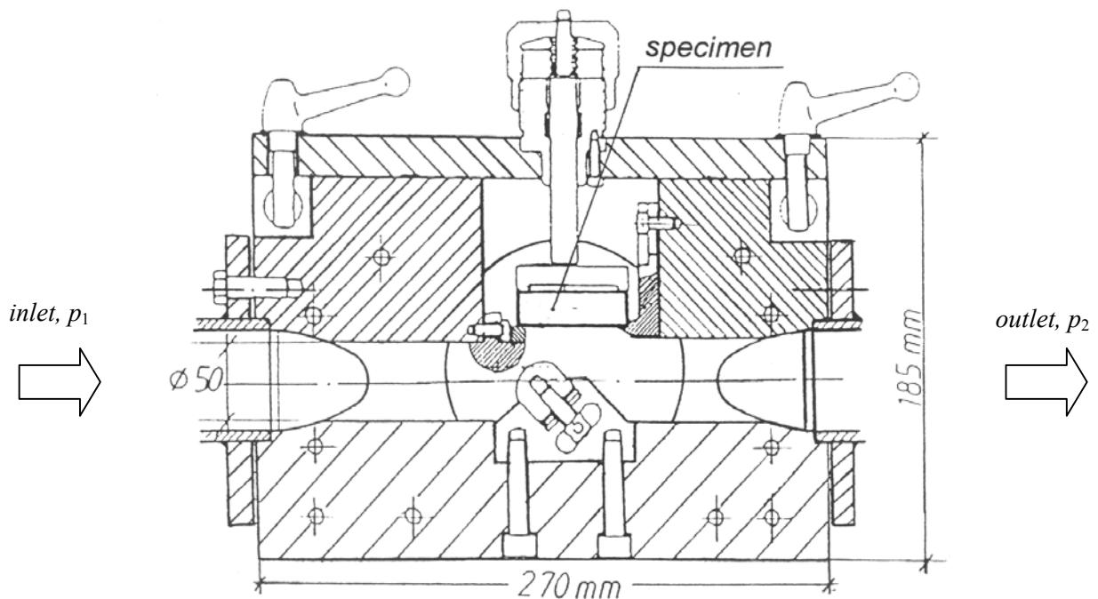
specimen width: 30 mm, height: 8 ... 12 mm, length: 60 mm
