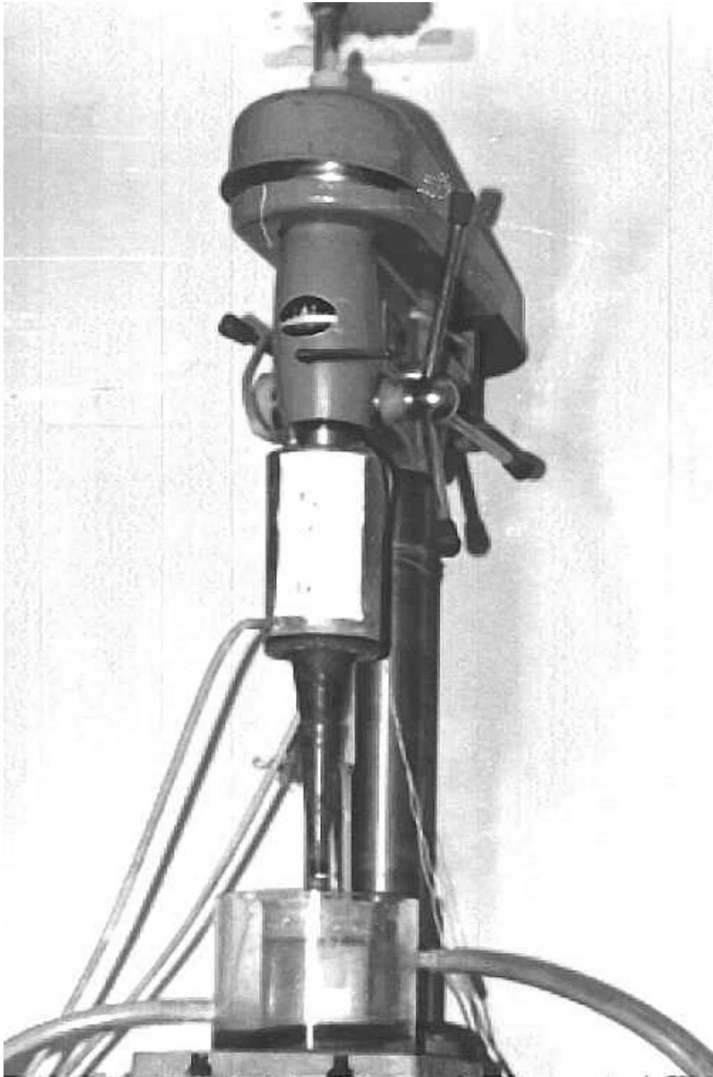
The Vibratory Cavitation Erosion Test Apparatus
