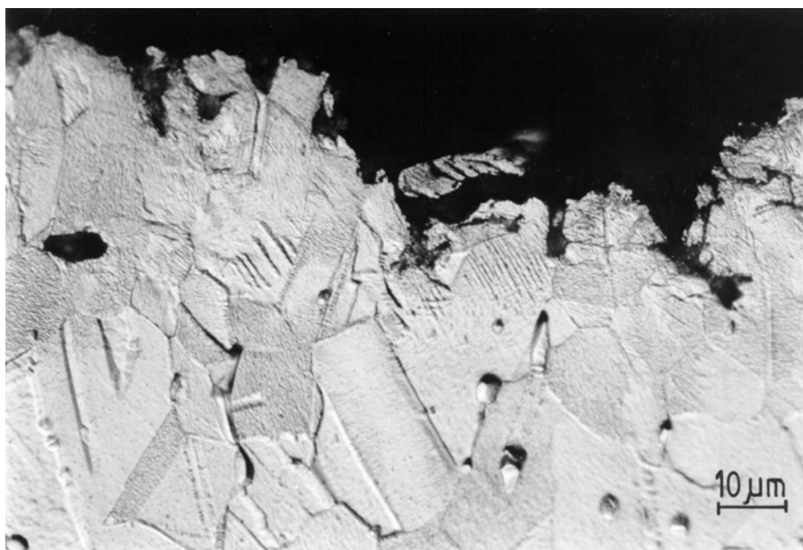
FIGURE 7 The cavitated edge
