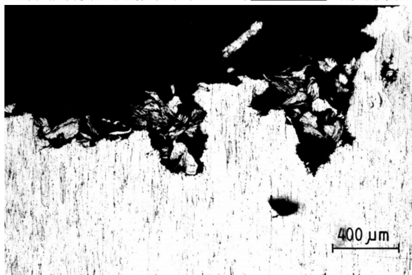
FIGURE 6 The cavitated edge at higher magnification
