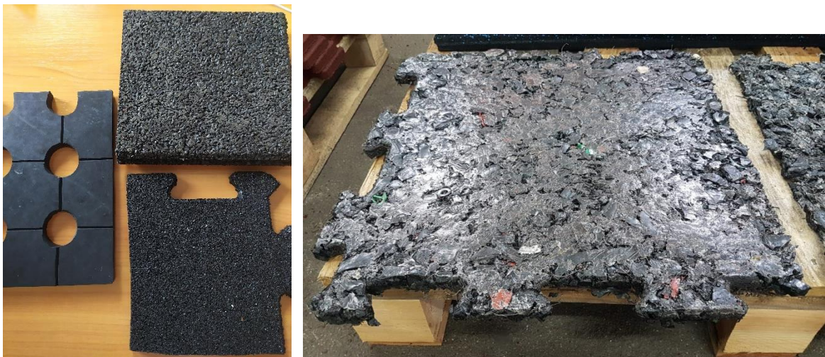
Fig. 3. Recycled rubber granulate products (left) and PLASTER Kuligowskiego® based on raw tire waste (right)
